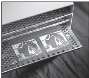
A dryer, such as the PB 500 (shown) with heated circulating air will significantly reduce drying time.
